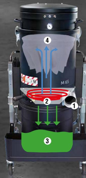
THE MATERIAL ENTERS THE CHAMBER FROM THE SUCTION INLET (1) AND THANKS TO THE CYCLONE (2) IT LOSES SPEED, SETTLING INSIDE THE VACUUM'S BIN (3). THIS WAY 90% OF THE MATERIAL IS CLEARED, GRANTING A LONGER LIFE FOR THE FILTER.
