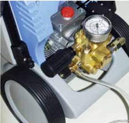
The oil level must be between the two markings on the oil dipstick.
