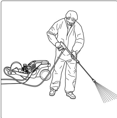
**13.** Ventilation of the machine: Pull and release the trigger several times.
